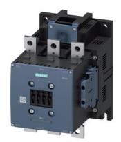
Power contactor, AC-3 300 A, 160 kW / 400 V AC (50-60 Hz) / DC operation 220-240 V UC Auxiliary contacts 2 NO + 2 NC 3-pole, Size S10 Busbar connections Drive: conventional screw terminal
