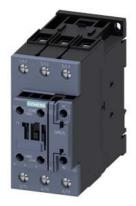
power contactor, AC-3 50 A, 22 kW / 400 V 1 NO + 1 NC, 230 V AC, 50 Hz, 3-pole, Size S2, screw terminal
