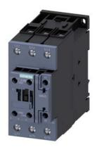
Contactor, AC-3, 37 kW / 400 V, 1 NO + 1 NC, 110 V AC, 50 Hz, 3-pole, Size S2, screw terminal
