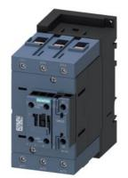
power contactor, AC-3 95 A, 45 kW / 400 V 1 NO + 1 NC, 230 V AC, 50 Hz 3-pole, 3 NO, Size S3 screw terminal
