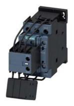
Capacitor contactor, AC-6b 25 kVAr, / 400 V 1 NO + 2 NC, 230 V AC, 50 Hz 3-pole, Size S0 screw terminal
