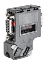
PROFIBUS bus connector, RS 485, screw, with programming port, 35° SIMATIC DP, Connection plug for PROFIBUS up to 12 Mbit/s with inclined cable outlet, 15.8x 54x 39.5 mm (WxHxD), terminating resistor with isolating function, With PG receptacle
