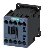
Power contactor, AC-3 9 A, 4 kW / 400 V 1 NC, 24 V AC, 50 / 60 Hz 3-pole, Size S00 screw terminal
