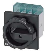
SENTRON, Switch disconnector 3LD, main switch, 3-pole, lu: 16 A, Operating power / at AC-23 A at 400 V: 7.5 kW, front-mounted, rotary operating mechanism, black, 4-hole mounting of the handle
