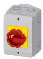
SENTRON, Switch disconnector 3LD, emergency switching-off switch, 3- pole, lu: 32 A, operating power / at AC-23 A 400 V: 11.5 kW, molded-plastic encapsulation for metric cable gland, rotary operating mechanism, red/yellow
