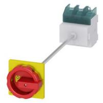
SENTRON, Switch disconnector 3LD, emergency switching-off switch, 3- pole, lu: 125 A, operating power / at AC-23 A 400 V: 45 kW, floor mounting with door coupling, rotary operating mechanism, Red / yellow, 4-hole mounting of the handle
