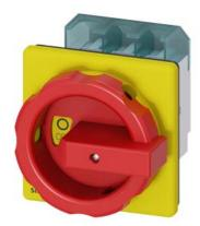
SENTRON, Switch disconnector 3LD, emergency switching-off switch, 3- pole, lu: 63 A, operating power / at AC-23 A 400 V: 22 kW, front-mounted, rotary operating mechanism, Red / yellow, 4-hole mounting of the handle
